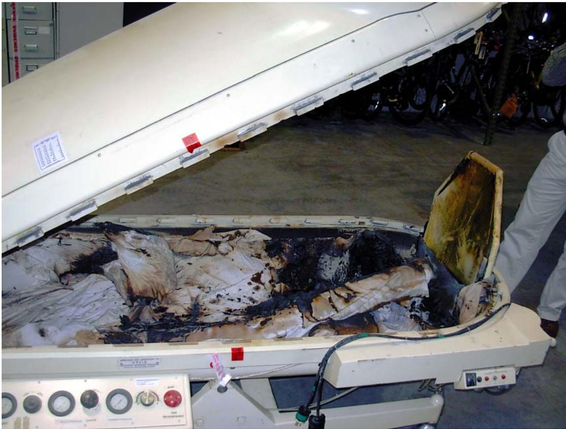
Figure 3: Interior of Vickers 'clamshell' chamber. Approximately  $\frac{3}{4}$  of the head end of the chamber interior is visible.
